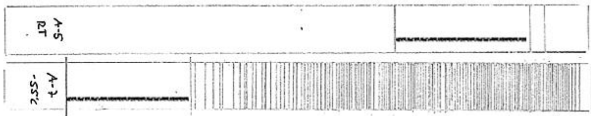
Figure 5. Test strip 5 and 7 of Hexcel material A; the bold stripe shows the distance in the jig to the first crack: A-5 room temperature test stopped with first sound of crack; penetrant indicates two cracks; A-7 cold temperature test at -55° pushed fully into jig resulting in a high crack density
