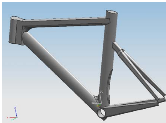
Figure 1. The Unigraphics 7.0(Siemens PLM Software, Torrance, CA, USA) CAD model of the bicycle frame in this study.
