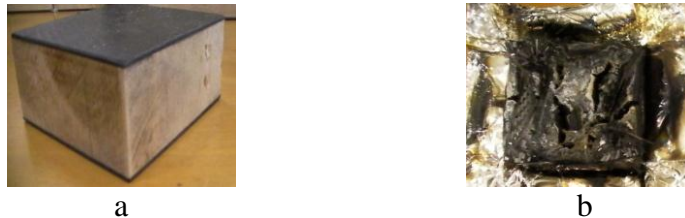
Figure 1. Sandwich composite, original (a), after cone calorimeter testing (b)
