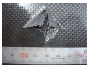
(d) 5wt% flexible interphase including 1.0 wt% of grafted CNTs
