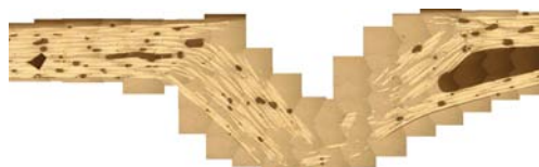
(c) 5wt% flexible interphase including 0.5wt% of grafted CNTs
