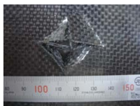
(c) 5wt% flexible interphase including 0.5wt% of grafted CNTs
