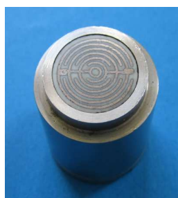
Figure 2: Reusable TMS comb sensor for the mold of the RTM process
