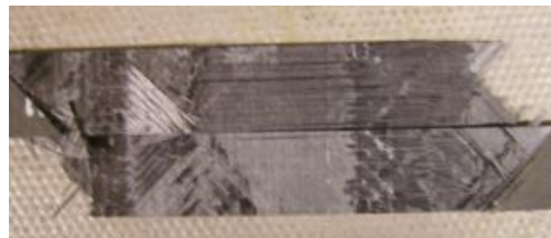
Figure 6. Mode B = Fibre pull out, (interlaminar and intralaminar failure) scarf angle 0.7° adhesive Redux 312
