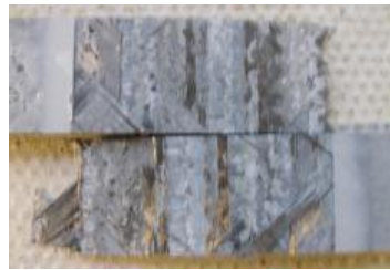
Figure 5. Mode A = Cohesive failure except on the 90° plies where fibre pull out is evident scarf angle 3° adhesive Redux 312
