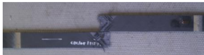
Figure 7. Net section failure (but at approx 50-60% of plain coupon failure load) scarf angle 0.7° adhesive EA9695 0.5 psf.
