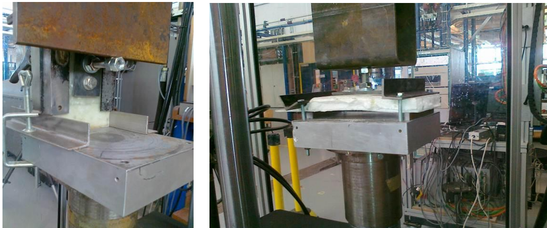
Figure 16. In-plane (left) and out-of-plane (right) testing of attachment points
