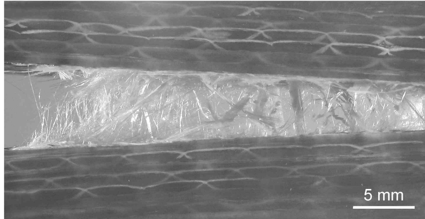
Figure 1. Photo of a glass fibre composite experiencing large-scale crack bridging.
