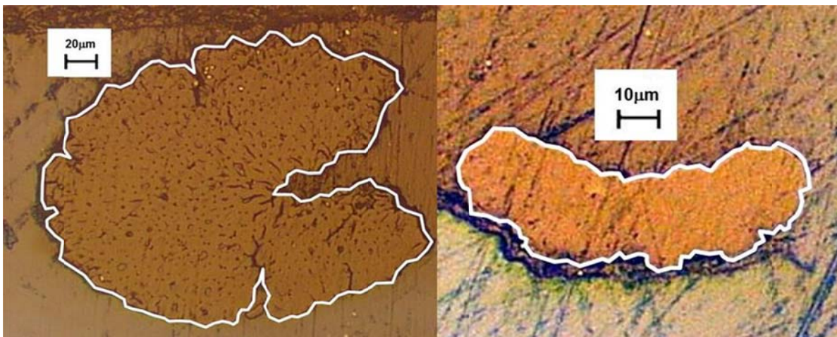
Figure 1. Cross section view of single Sisal and Flax fibre
