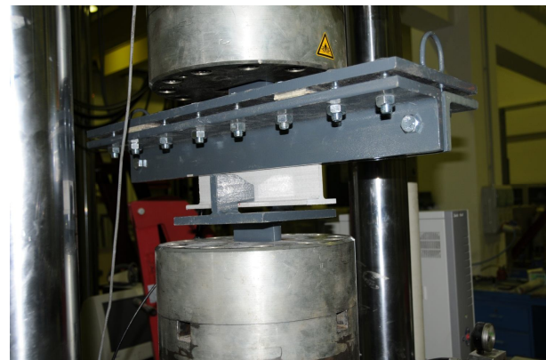
Figure 2. Mid Point Pull-Out Test Setup.
