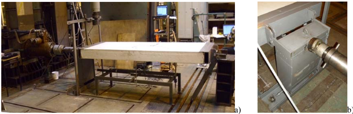
Figure 4. Buckling tests of SIPs: a) experimental set-up, b) support
