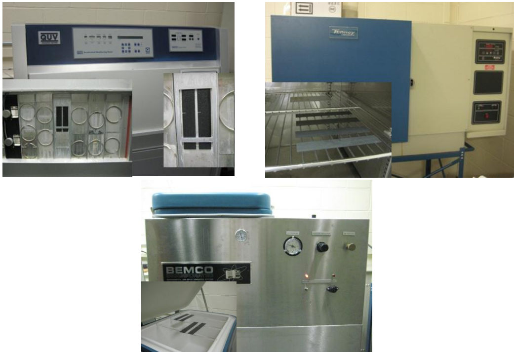
Figure 1. Environmental exposure performed in the laboratory with accelerated aging chambers, Top left, QUV/se ultraviolet radiation and condensation chamber, Top right, Tenney BTR5 temperature and humidity chamber, Bottom, Bemco P700XL salt spray. Insets show composite samples in chambers.
