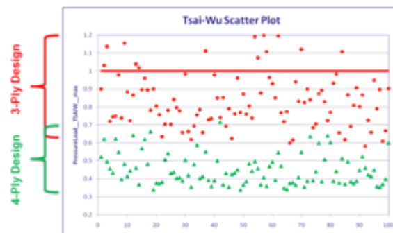
Figure 9. Scatter plot showing the robustness and reliability of the 3-ply and 4-ply designs.
