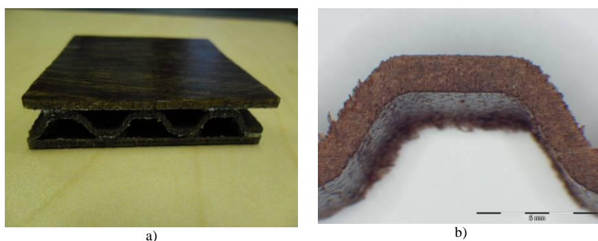
Figure 2. a) Manicaria/PLA core sandwich specimen. b) half-hexagonal cell walls
