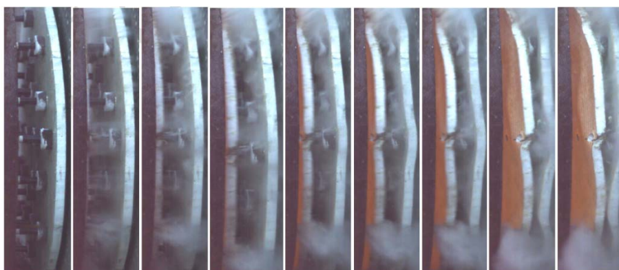
Figure 8. Progressive crushing stages of the 25 composite tubes (25 numbers) for 150 g of C4.
