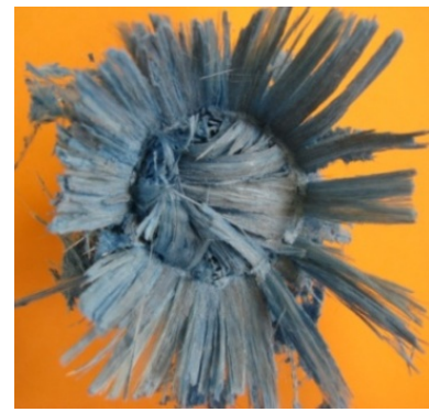
(c) Deformation pattern of commercially available pultruded GFRP composite tube (2 mm wall thickness) with triggering type 2 for 40g of C4 with 15 cm stand-off distance.
