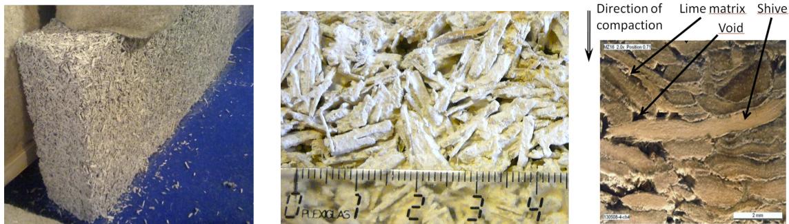
Figures 1, 2 & 3: 1: Example of HLC breezeblock, 2: Random distribution of shives embedded in lime within HLC before compaction (measure in cm), 3: Micrograph of shives within a compacted HLC (cross section).
