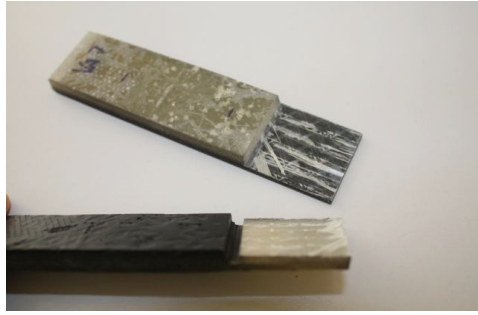
Figure 8. LFT failure mode for the joint VA-07
