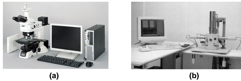
Figure 1. Image analysis workstations: (a) optical microscope Nikon ME600 Eclipse (b) scanning electron microscope VEGA-TESCAN
