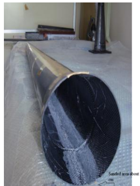
Figure 4. Grounded side of the tail cone.
