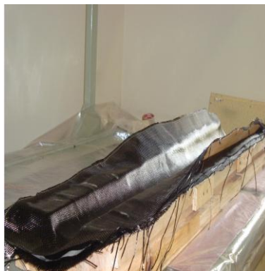
Figure 1. Production of tail cone by using hand lay-up technique.
