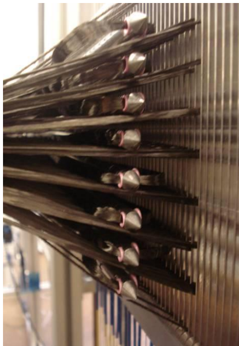
Figure 4: multi-shed weft insertion
