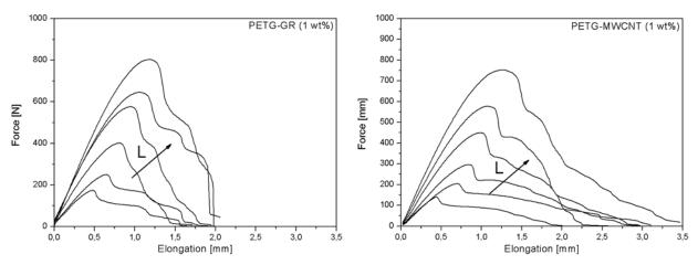
Figure 2. F-x traces as a function of the ligament length (L) measured on DEN-T specimens of PETG-GR (a) and PETG-MWCNT (b).
