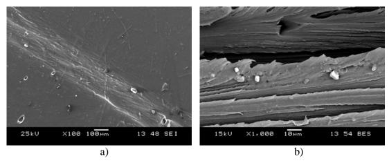
Figure 7. SEM pictures from the surface of the transition between the plastic zone (bottom left) and bulk (top right) (a) and from the fracture zone (b) of a DEN-T specimen of PETG-BA
