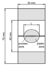
Figure 1. Schematic diagram showing the fracture zones in a DEN-T specimen
