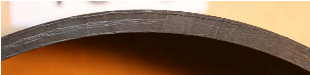
Figure 15: Interlaminar shear failure of an 8 ply specimen with a 4 ply crease
