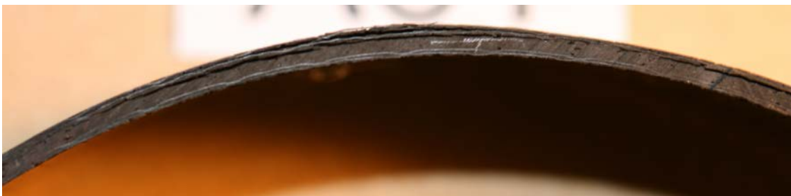
Figure 13: Interlaminar shear failure of an 8 ply control specimen
