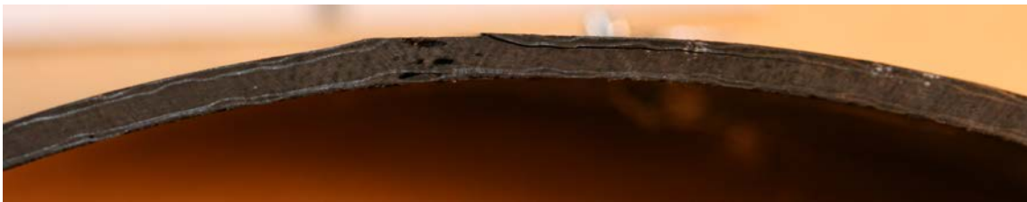
Figure 10: Interlaminar tensile failure of an 8 ply specimen with a 4 ply crease
