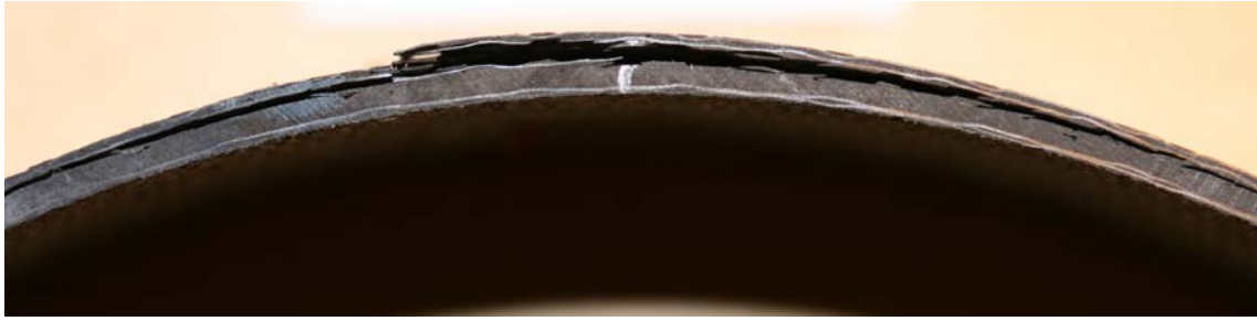
Figure 6: Interlaminar tensile failure of an 8 ply control specimen
