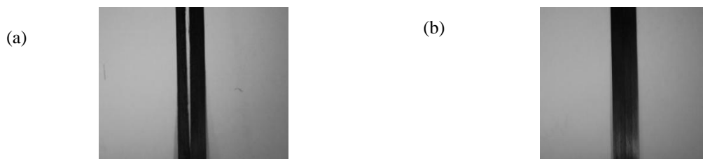
Figure 3. Carbon fibre T700/IM7 hybrid reinforced PA-12 composite tape manufactured (a) without and (b) with commingling process
