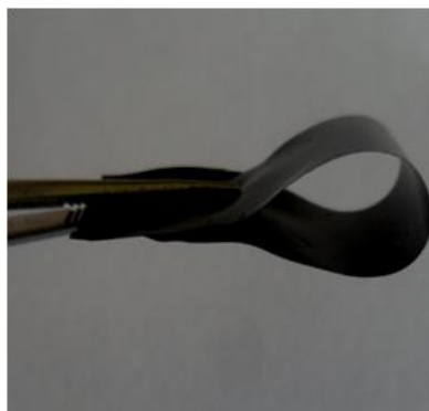
Figure 1. Optical images of nanocellulose based composite film containing 20 wt.% PANI after bending by 180°, with thickness of 50µm
