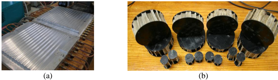
Figure 1. Sandwich panel manufacturing (a) Matched-die used for forming (b) Sandwich panels for acoustic test (diameters of 100mm and 30mm)
