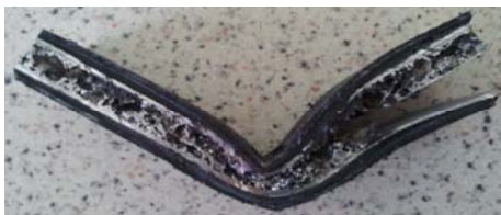
Figure 4. GFR-AFS Alulight panel collapsed after bending test ( L = 55 mm).
