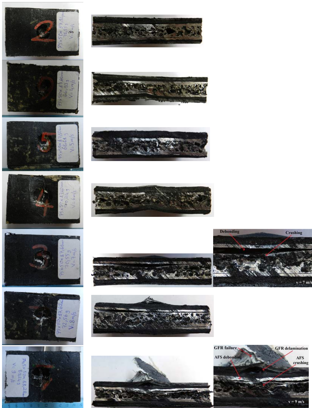
Figure 11. Damaged GFR-AFS panels after impact tests.
