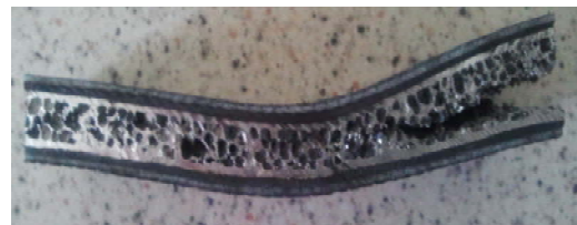
Figure 7. GFR-AFS Schunk panel collapsed after bending test ( L = 125 mm).
