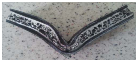
Figure 6. GFR-AFS Schunk panel collapsed after bending test ( L = 55 mm).
