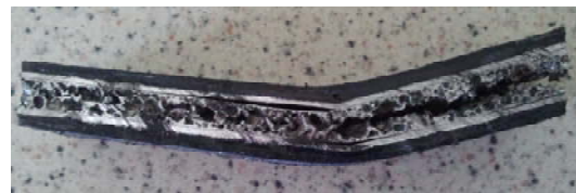
Figure 5. GFR-AFS Alulight panel collapsed after bending test ( L = 125 mm).
