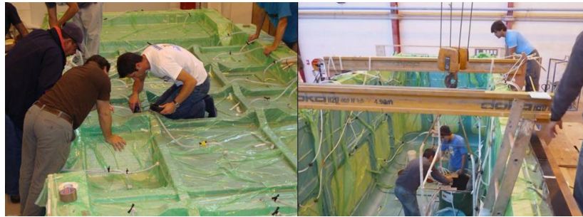
Figure 2 – Infusion of the parts using open moulds
