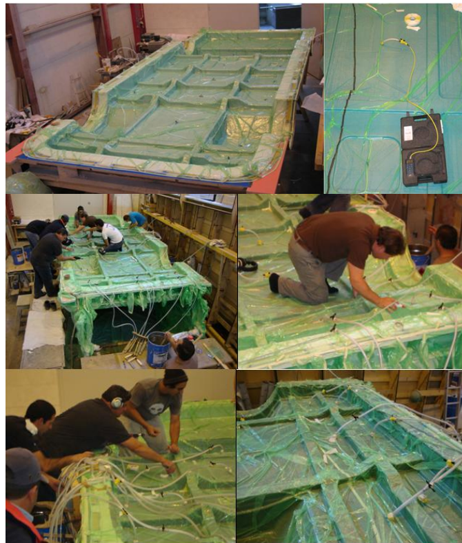
Figure 5 –Vacuum bag placement, pressure control and infusion (Floor)
