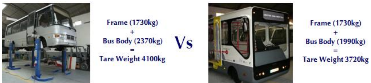
Figure 6 – The weight reduction achieved on the Bus bodywork was 380kg (around 16%)
