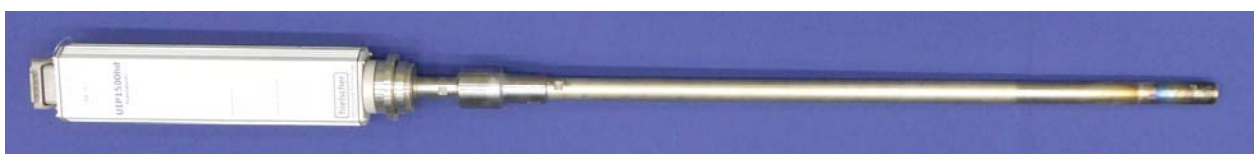
Figure 1. Ultrasound generator (left) with attached booster and sonotrode
