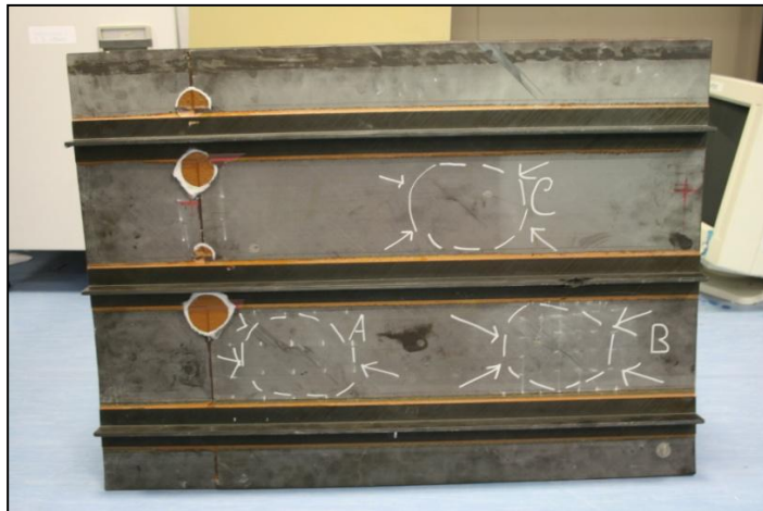
Figure 6. Stringer panel (back side view) with 3 impacted areas
