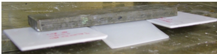
Figure 6. Deflection of the PLA (middle) and PLA/Mg-80°C specimens (left and right) at 120°C
