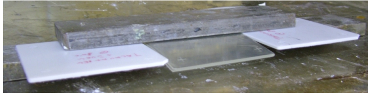
Figure 4. Deflection of the PLA (middle) and PLA/Mg-80°C specimens (left and right) at 60°C
