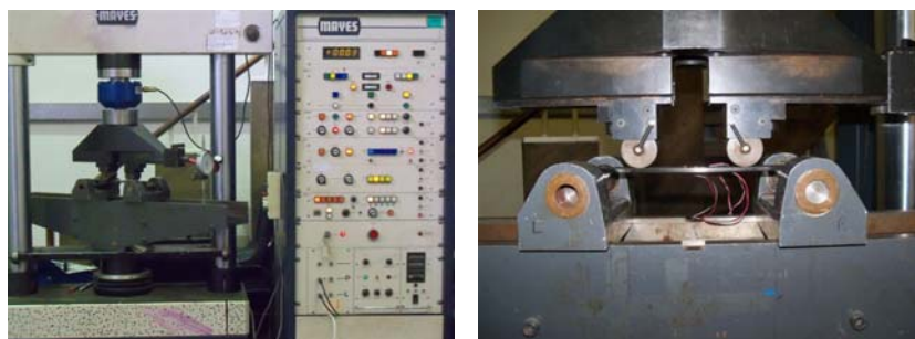
Figure 1. Servo-electric universal machine used in the tests and specimen instrumented and mounted.
