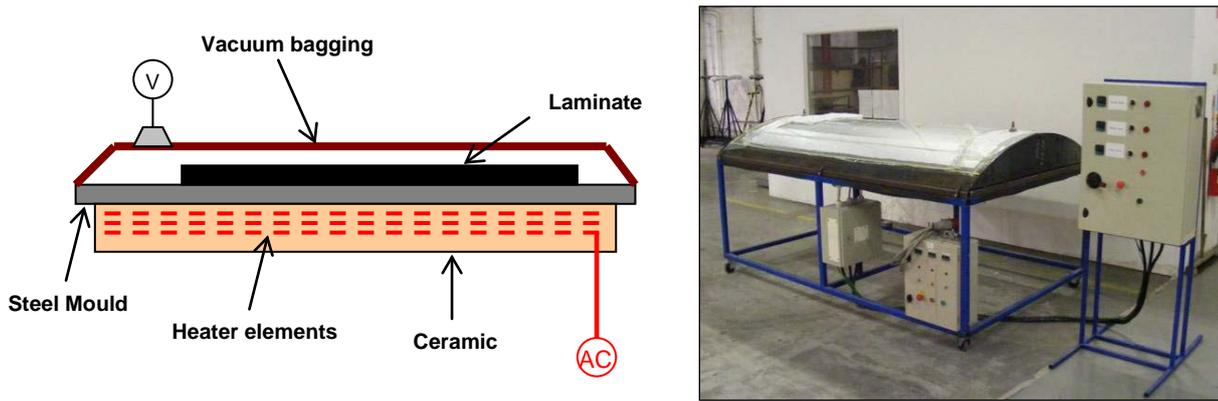
**Figure 3:** Schematic of MECH<sup>TM</sup> Tool and demonstrator tooling
