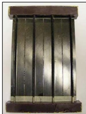
**Figure 9:** Multi-stiffened test panel
