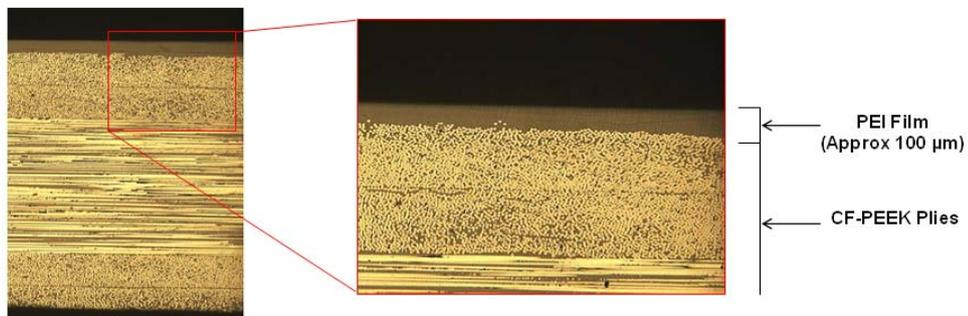
**Figure 8:** Cross-section through laminate showing PEI film layer
