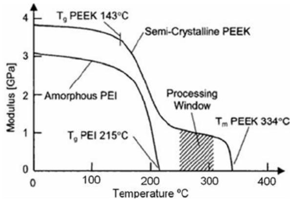
**Figure 7:** Process window for Amorphous Interlayer Bonding [5]
