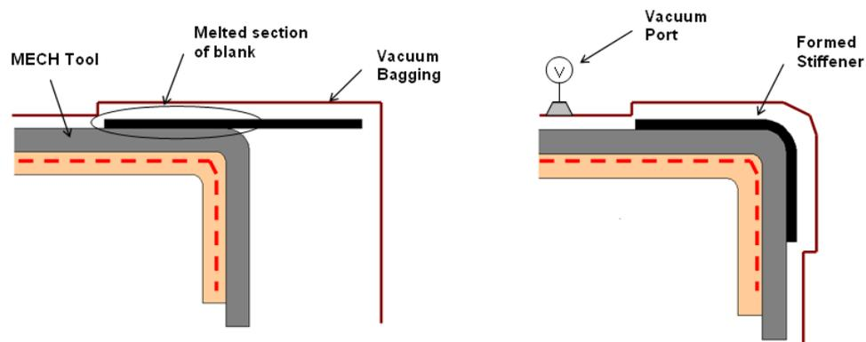
**Figure 5:** (Left) Stiffener blank is positioned overhanging on MECH<sup>TM</sup> Tool
