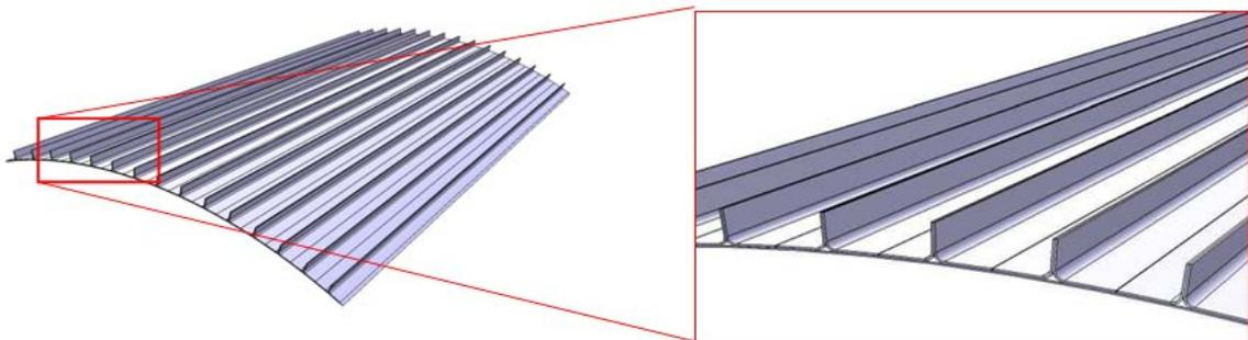
**Figure 2:** Re-designed configuration; base panel with bonded T-section stiffeners
