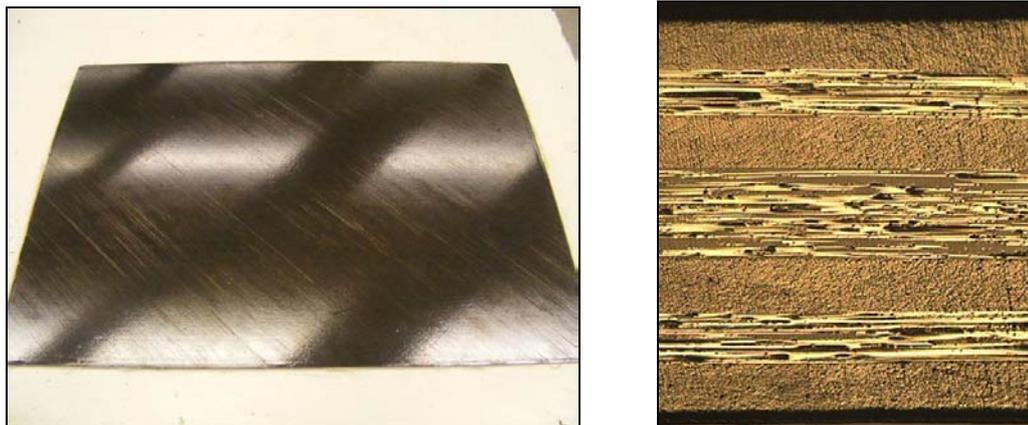
**Figure 4:** OOA CF/PEEK laminate and micrograph (x30 mag)
