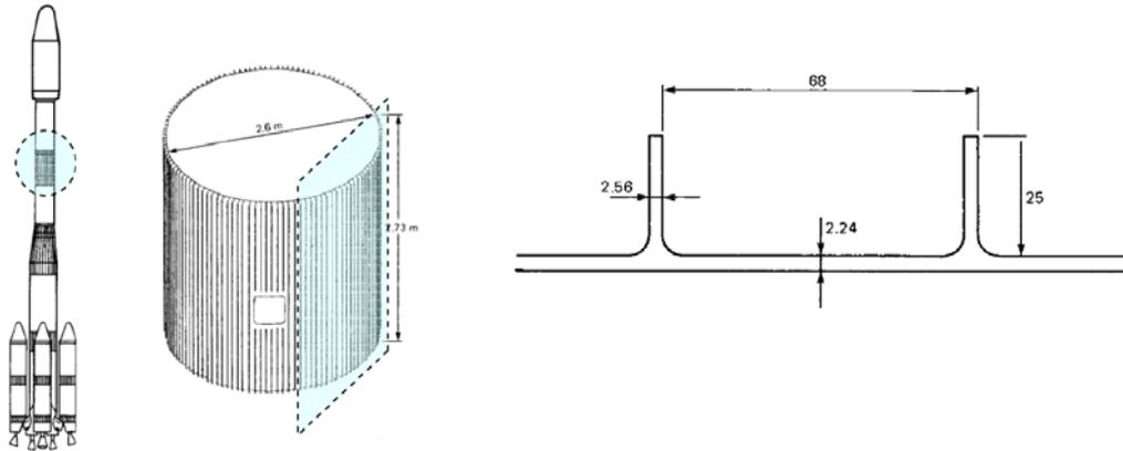
**Figure 1:** Detail view of original Ariane 4 2/3 interstage
