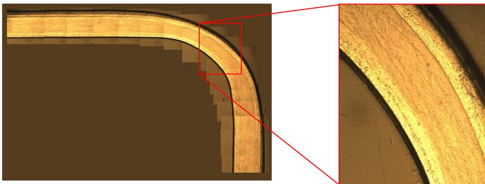
**Figure 6:** Micrograph of formed L-section stiffener radius
