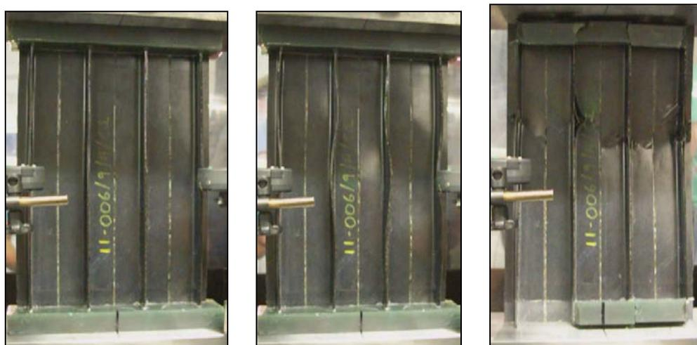
**Figure 11:** Images of panel at 240 kN, 250 kN and 265 kN (respectively)
