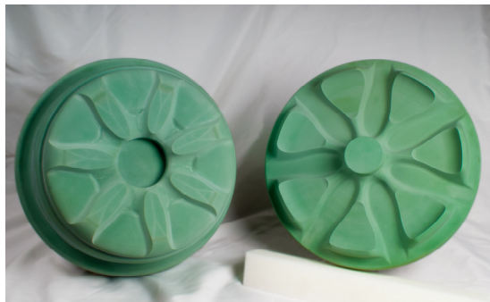
Figure 6. Moulds made of closed cell rigid foam with polyurethane base for manufacturing the prototype wheel.
