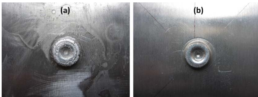
Figure 4. The deformed sheet at the bottom of the rivet: (a) damaged for '24h-340' joints; (b) sound for '24h-280' joints.
