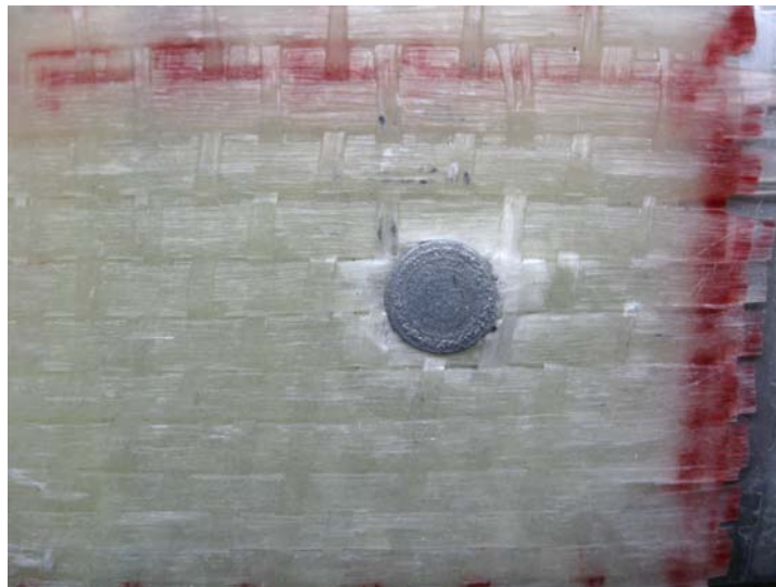
Figure 3. Delamination at the substrates interface of '24h-340' joints.
