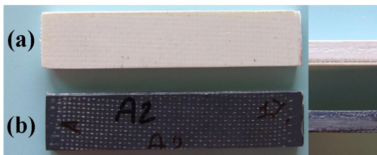
Figure 6. Sandwich structures based on Neat PEN (a) and the 1.0% EG filled matrix (b)
