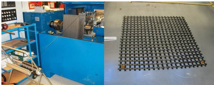
Figure 2. Winding of preform in tool. Towpreg grid ready for infusion.
