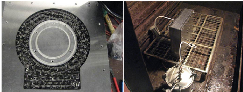
Figure 9. Top flange of towpreg loaded tool. Isothermal pressure casting at 45 °C.
