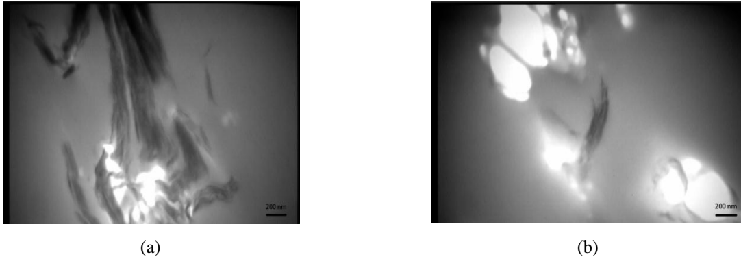
Figure 1. TEM images of PF/clay nanocomposites at 2.5 wt%. a) PF/CN b) PF/CB.
