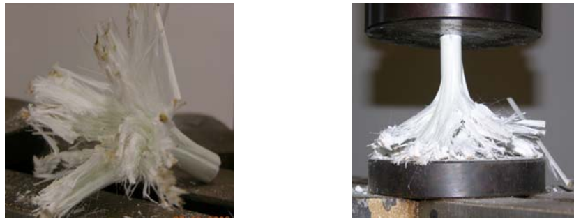
Figure 1. Compression of a traditional GFRP bar
