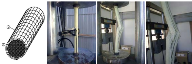
Figure 3. Configuration and compression test of RTHp bar
