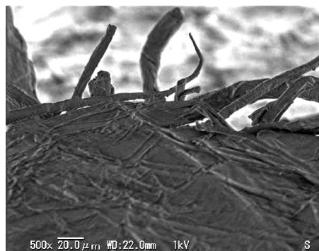
Fig.5 SEM photograph of the broken surface of 23 wt% bamboo reinforced onion composite
