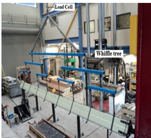
Fig.8-Static Loading Through of Whiffle Tree System Fig.9- Dynamic test of FRP Tower Segment
