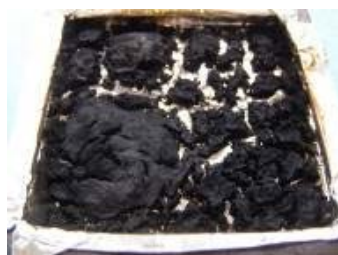
Figure 6. PLA/clay nanocomposites residue obtained after cone calorimeter experiment
