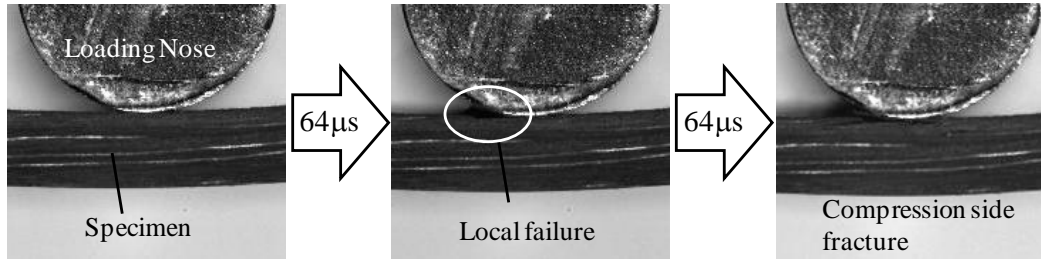
Figure 7. Instant images of flexural fracture of hybrid laminate.
