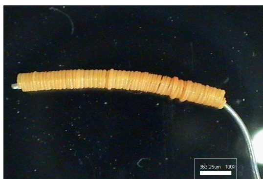
Figure 4. Photographs of coils made of s-PVA composite fibers.
