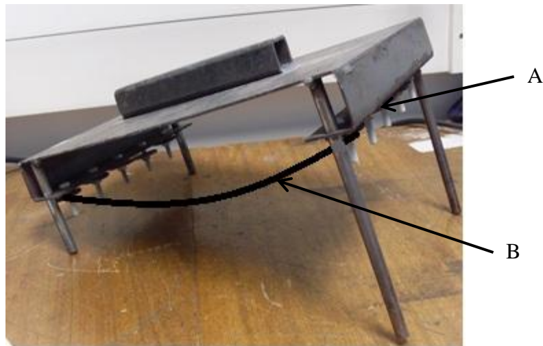
Figure 1. Image of the steel rig used for bundled TC.
