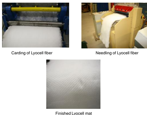
Figure 3. Carding and needling of Lyocell fiber to achieve a non-woven fiber mat
