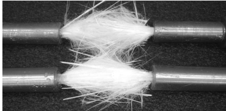
Figure 5. View of destroyed unidirectional fiberglass specimens after low temperature uniaxial tension
