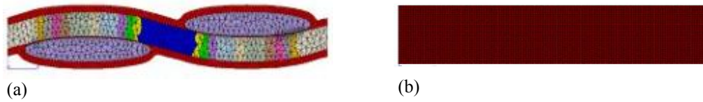
Figure 6. (a) RVE meshing cell, (b) homogeneous equivalent model.
