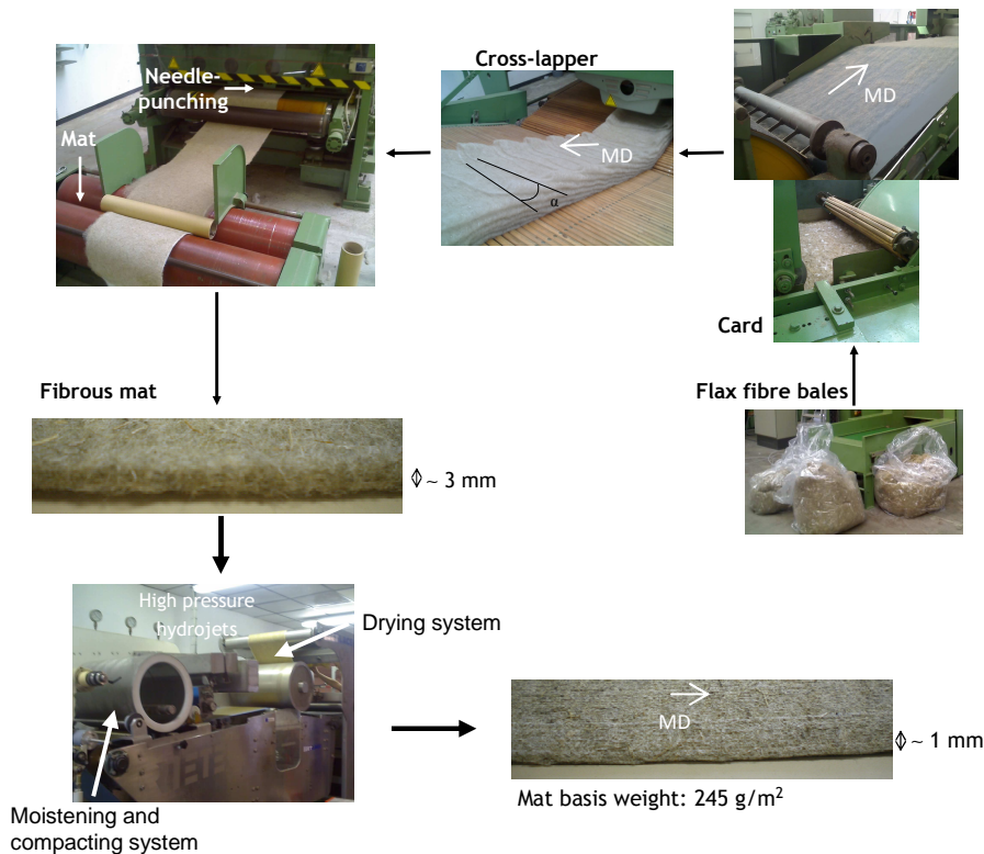
Figure 1. Schematic description of the production process of the needed flax fibre mats.
