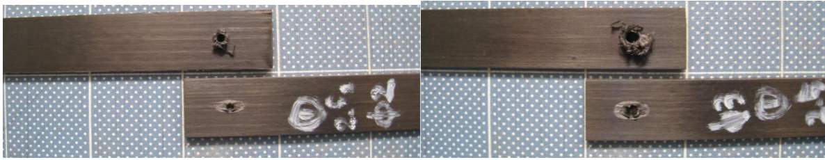
Figure 12. Joint part of single lap specimens by spot welding (UD): (left) oscillation time of 2.5 sec with horn diameter of 2 mm; (right) oscillation time of 2.5 sec with horn diameter of 3 mm.
