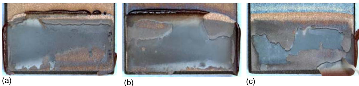
Figure 13. Fracture surface of laser treated surface at the initial state (a) and after exposure to 80°C deionized water of 7 days (b) and 17 days (c)
