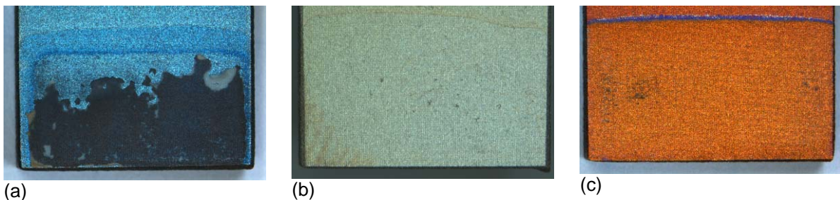
Figure 12. Fracture surface of samples anodised in 5M NaOH electrolyte (a), in 1M H 2 SO 4 electrolyte (b), and in 1M H 3 PO 4 electrolyte (c) after exposure to 80°C deionised water
