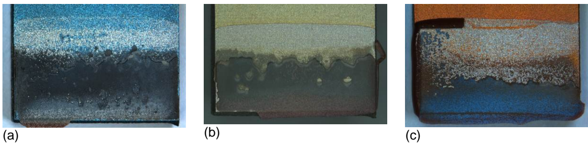
Figure 9. Fracture surface of samples anodised in 5M NaOH electrolyte (a), in 1M H 2 SO 4 electrolyte (b), and in 1M H 3 PO 4 electrolyte (c) at the initial state
